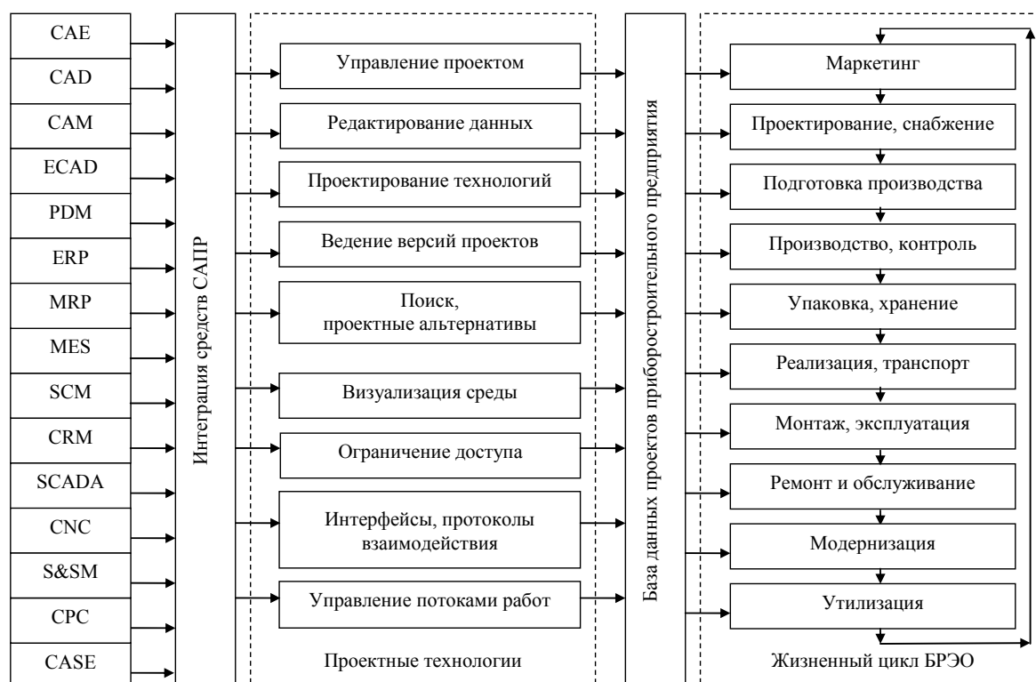
Рис. 1. Функциональная схема взаимодействия разнородных средств САПР в составе единой отраслевой САПР поддержки жизненного цикла БРЭО (CAE – Computer Aided Engineering; CAD – Computer Aided Design; CAM – Computer Aided Manufacturing; ECAD – Electronic Computer Aided Design; PDM – Product Data Management; ERP – Enterprise Resource Platting; MRP – Manufacturing Requirement Platting; MES – Manufacturing Executing System; SCM – Supply Chain Management; CRM – Customer Relationship Management; SCADA – Supervisory Control and Data Acquisition; CNC – Computer Numerical Control; S&SM – Sales and Service Management; CPC – Collaborative Product Commerce; CASE – Computer Aided Software Engineering)
